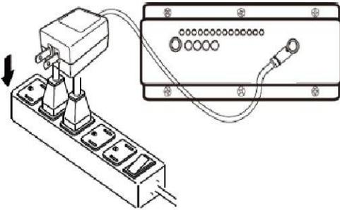
2. The power status LEDs will blink to indicate the capacity of battery when the device is in charge mode. When the battery is at full charge the 4 LEDs should all be ON.
