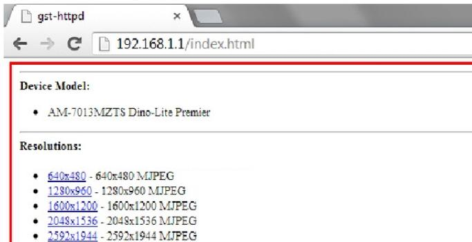
6. Select the desired resolution from the list. Please note that frame rates will decrease as resolution increases. Video will begin streaming once a resolution has been chosen. (The device supports 640x480 resolution. Additional resolutions are available when using 5MP Dino-Lite models.)
